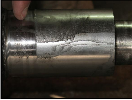
Degradation of the hard chrome on the axle.
