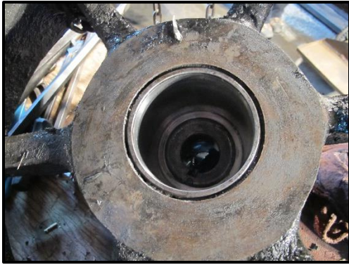
The inside of wheel with cage bearing removed. (Thanks to Nicholas, the town bicycle mechanic, who spotted the retaining ring on the seal.)
