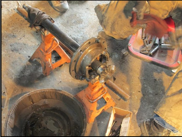
The internal gear that is part of the spider gear.
