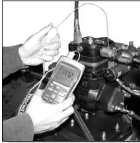
Testing the temperature at the discharge fitting.
