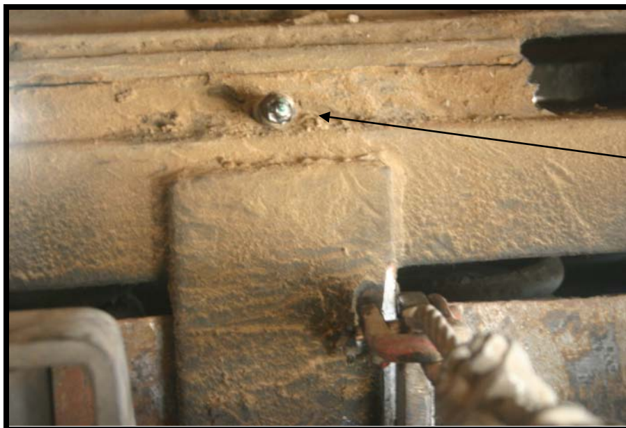
Zerk Fitting on Power Truck (Look for 2 - Front and back of truck)
