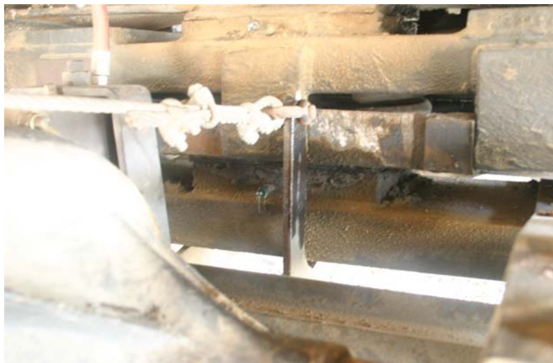
Hand Brake Cable with air can behind.
