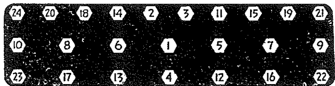
Fig. 2 Head tightening chart for 213 and 230 engines
